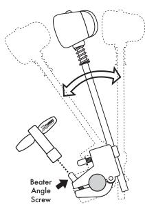
The Beater of the Dyno-Matic Pedal can be positioned independently - without affecting the positions of the Pedalboard, the Spring Arm, or the Axle height. The forward, or backward angle of the Beater Cam is adjusted by loosening the Beater Angle Screw with the Drum Key, as shown on the left. The length of the Beater shaft can be changed by loosening the Beater Length Screw with the Drum Key, as shown on the right. Be sure to tighten the screws securely once
