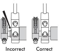
The Beater Cam should be centered on the knurled axle bushing.
